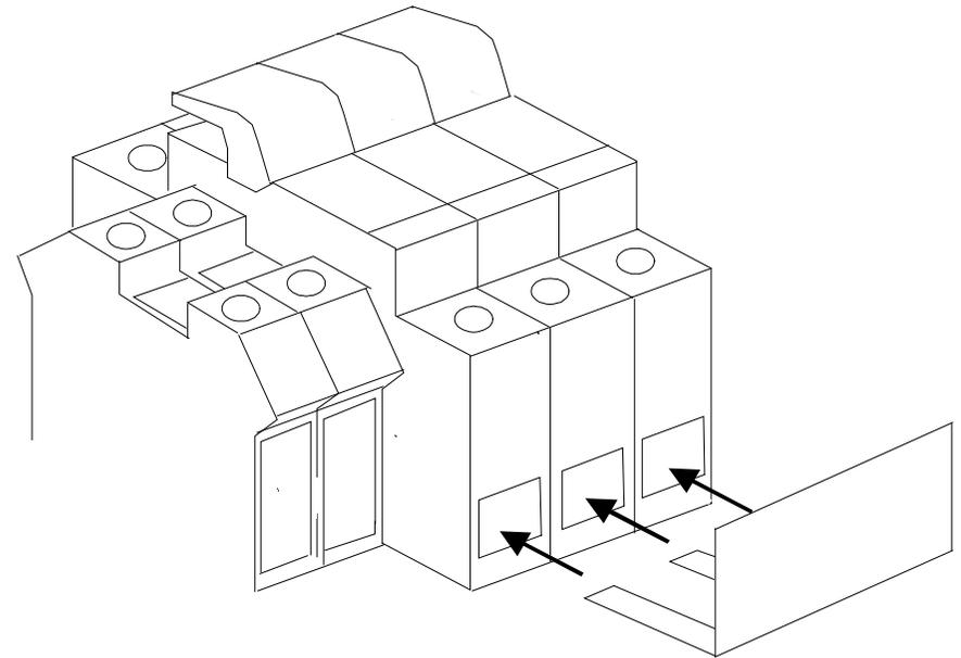
re-connected to a 3-phase supply then the link **MUST** be removed.
