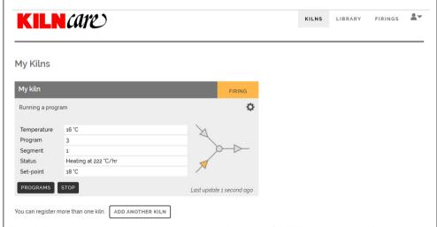
If the kiln is already running when you log into the GATEway then the first screen will give the status of the kiln, whether it is heating or cooling, the program
