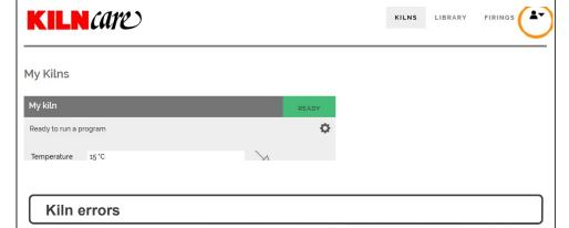
In the event of the kiln developing a fault or a fault in the process causes the controls internal protection triggers to kick in and turn the kiln off, then the GATEway will show you that the firing has stopped (see below) and it will also tell you the error code number. This can then be cross checked with your controller manual to find out what exactly has caused the problem.
